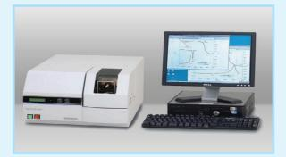
2. Oxidation and\or Combustion: The simplest materials characterization is the residue remaining after a reaction. The thermogravimetric analyzer would combustion the sample by heating it beyond the ignition temperature of a sample. The resultant TGA curve plotted with the y axis as percentage of initial mass would show the residue at the final point of the curve. Oxidative mass losses are the most common observable losses in TGA.
