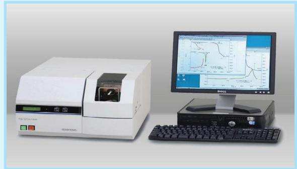
**2. Oxidation and/or Combustion:** The simplest materials characterization is the residue remaining after a reaction. The thermogravimetric analyzer would combustion the sample by heating it beyond the ignition temperature of a sample. The resultant TGA curve plotted with the y axis as percentage of initial mass would show the residue at the final point of the curve. Oxidative mass losses are the most common observable losses in TGA.
