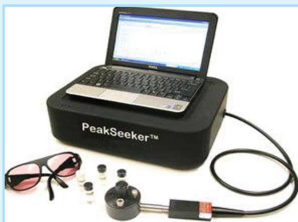
**Introduction:** Raman spectroscopy is used to observe vibrational, rotational, and other low-frequency modes in a system. Raman spectroscopy is commonly used in chemistry to provide a structural fingerprint by which molecules can be identified.
