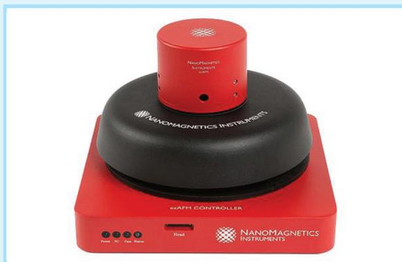
**Introduction:** AFM is a type of scanning probe microscopy (SPM), with demonstrated resolution on the order of fractions of a nanometer, more than 1000 times better than the optical diffraction limit. The information is gathered by "feeling" or "touching" the surface with a mechanical probe. Piezoelectric elements that facilitate tiny but accurate and precise movements on (electronic) command enable very precise scanning.
