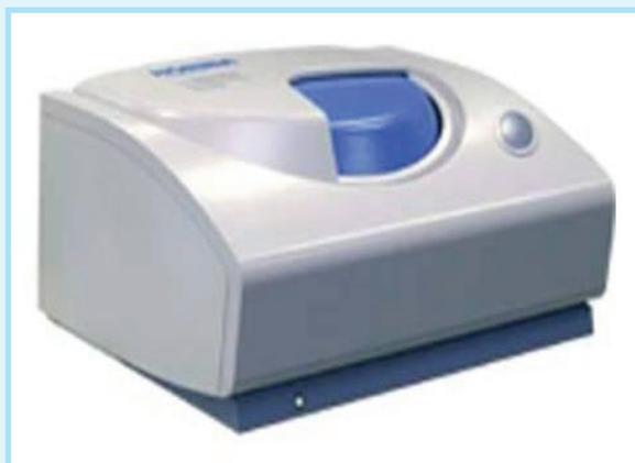
presence of large, unwanted particles. The upper limit is influenced by the density of the sample since DLS is modeled on all motion coming from Brownian motion, not gravitational settling.
